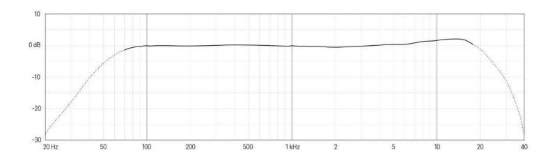
Typical on-axis response of a 2017 measured at 60 cm (23.6 in)
